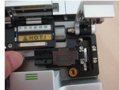
4. Clean the fiber, cut the fiber with fixed length on the cleaver of the machine.
