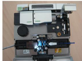
8 Put on welding joint with the fixture into specified location of the fusion splicing machine.
