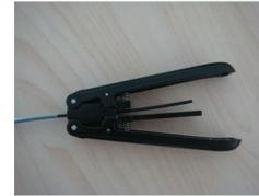
2. Put the cable into the stripping vice. The end of the cable should meet the mark. Press the handle and draw out the cable.
