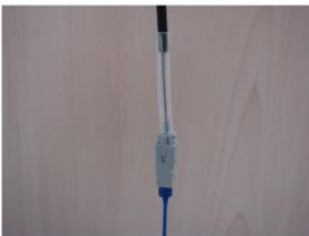
11 Push the shrinkable tube to the end of the welding joint carefully.
