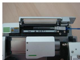
12 Put the welding point with the fixture into specified location of the fusion splicing machine.
