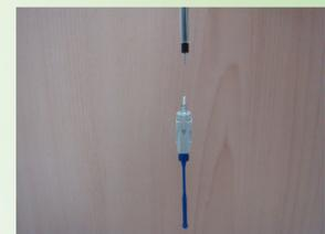
10 After the fusion, take out the welding joint and fiber carefully. And keep them vertical.
