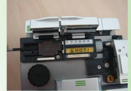
3. Fix the cable into the fixture, put the fixture into the fusion splicing machine to strip the 0.25mm coating with the stripper on the machine.
