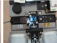
5. Put the fiber with fixture into the fusion splicing machine.
