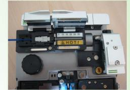
6. Fix the welding joint into the fixture, then put it into the fusion splicing machine to strip the cable.
