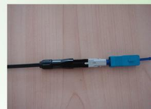
14 Push the boot to the welding joint. Screw the screw cap.
