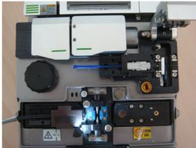
7 Clean the fiber. Put the welding joint with the fixture into the cleaver of the fusion splicing machine to cut the fiber.
