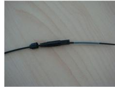
1. Penetrate the cable through the screw cap, boot and shrinkable tube one by one.
