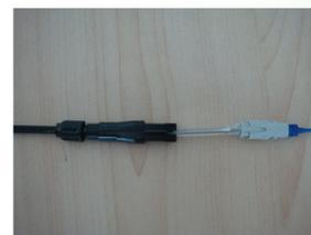
13 After fusion, take out the connector. Cool down for 5-10 seconds.
