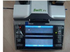
9 Close the cover of the machine. Then press the fusion key to melt.
